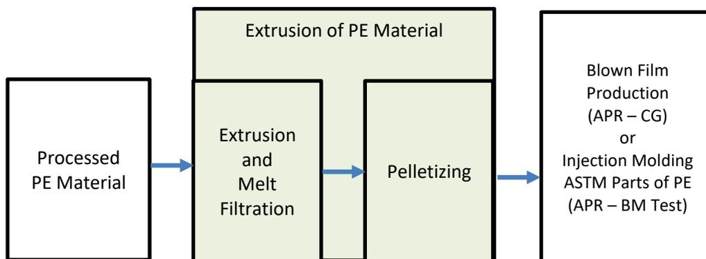
Note: There are situations in laboratory recycling assessments where it is necessary to add a heat history to PE resin to simulate a molding operation. This Extrusion Practice can be followed to add a heat history to PE samples – flake or pellets. Melt filtration and pressure measurement is not necessary when the practice is used only to add a heat history.
