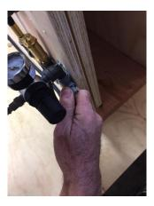
5. Connect the compressed air system to the compression device.
