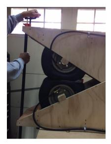
17. Open the compression device and remove the test article.
