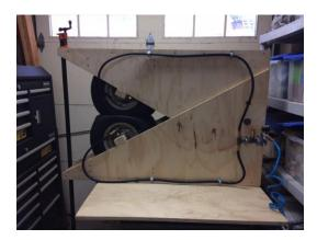
10. While pulling down on the compression device and top of pipe clamp, slip the bottom moving jaw of the pipe clamp as close to the other jaw as possible.
