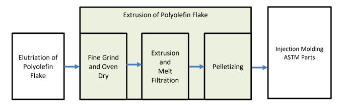
Note: There are situations in laboratory recycling assessments where it is necessary to add a heat history to polyolefin resin to simulate a molding operation. This Extrusion Practice can be followed to add a heat history to polyolefin samples – flake or pellets. Melt filtration and pressure measurement is not necessary when the practice is used only to add a heat history.
